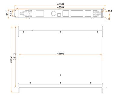
Tolerance: ±0.3 Unit: mm
